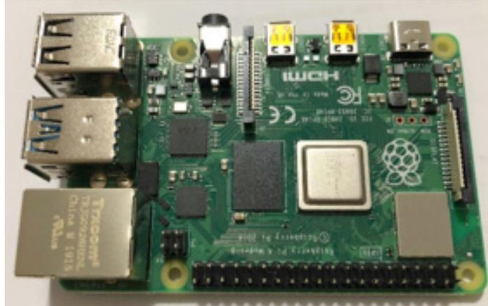
**Figure 4.** *Raspberry Pi 4 model B*
